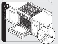
Remove pins from hole in hinges.
